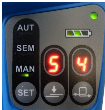
Li-Po storage battery half-full
