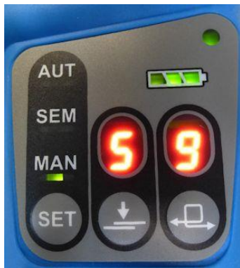
Li-Po storage battery fully charged
